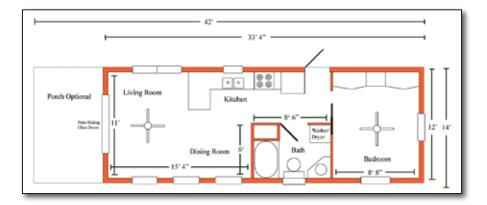
Example of a common floor plan used in the construction of our cabins. Additional floor plans as well as custom designs are also available.
